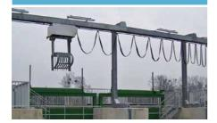
A screen is a hydraulic steel structure that is generally allocated at the intakes upstream of mills or hydroelectric power plants in order to collect debris and prevent damage to downstream turbines.
