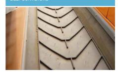
Belt conveyors offer cost-efficient conveying for a wide range of bulk materials at high feed rates for long and short distances. The endless conveyor belt used as a transport means is allocated on rollers for operation with relatively low power consumption, very low noise and minimal wear.
