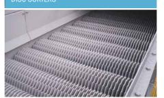
Disc sorters are mainly used to sort oversize particles out of an unclassified flow of bulk materials. They are used to protect downstream system parts from large impurities or to separate materials into fractions with a larger grain size.
